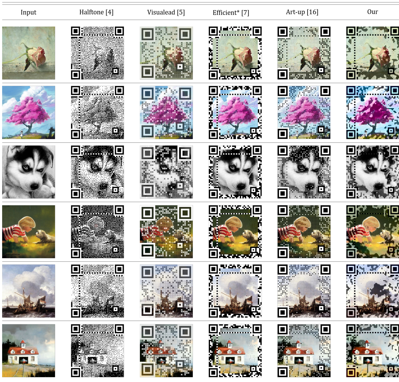
Fig. 22: Visual comparison of aesthetic QR Codes generated using different methods. Mark * means that the results of [7] are re-produced by ourselves.
